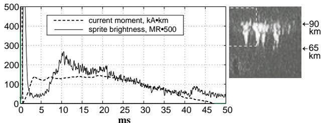
**Figure 5.** The extracted current-moment and sprite brightness waveforms, time-aligned as at the source, for the 07:17:38.767 sprite. The inset shows a video image of the sprite and the outline of the field-of-view of the photometer.
