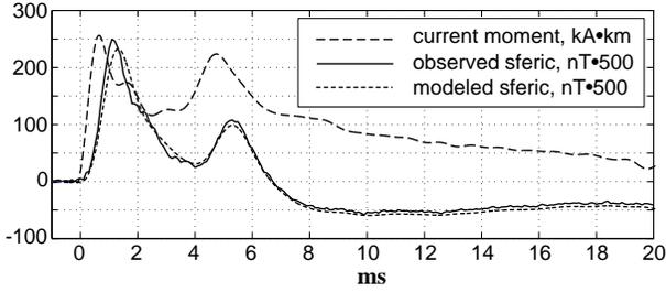
**Figure 2.** The extracted current-moment waveform, the observed ELF sferic in nanotesla (nT), and the modeled ELF sferic for the 07:48:36.682 sprite.
