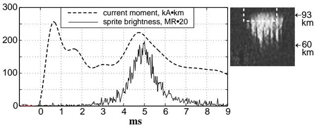
**Figure 3.** The waveforms for the extracted current-moment and sprite brightness in MegaRayleighs (MR), time-aligned as at the source, for the 07:48:36.682 sprite. The inset shows a video image of the sprite and the outline of the field-of-view of the photometer.
