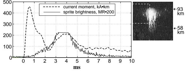
**Figure 4.** The extracted current-moment and sprite brightness waveforms, time-aligned as at the source, for the 07:08:41.020 sprite. The inset shows a video image of the sprite and the outline of the field-of-view of the photometer.
