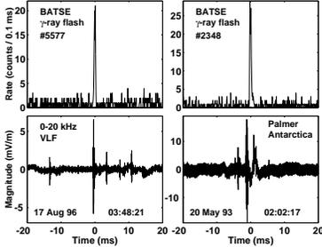
Fig. 1: Sample  $\gamma$ -ray recordings from a TGF (top) and associated VLF radio signatures of lightning (bottom)
