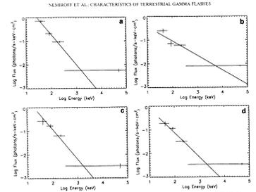
Fig. 2: TGF photon spectra approximated from BATSE's four energy channels [Nemiroff et al, JGR, 1997]
