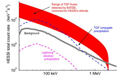
Fig. 8: Predicted HESSI count rates. Background courtesy of D. Smith. LEP flux courtesy of D. Lauben.
