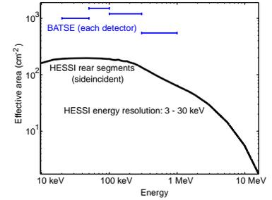
Fig. 7: Effective area and spectral resolution of BATSE LAD's and HESSI.
