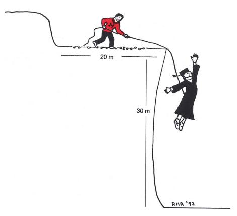
Substituting in the expressions for  $a_{1P}$ ,  $a_{2S}$ ,  $a_{2P}$ , and  $a_{3S}$ , and solving the system of four equations for F, we get a quadratic equation with a unique permissible solution of  $F = 2\mu mg$ ; our assumption stands.
